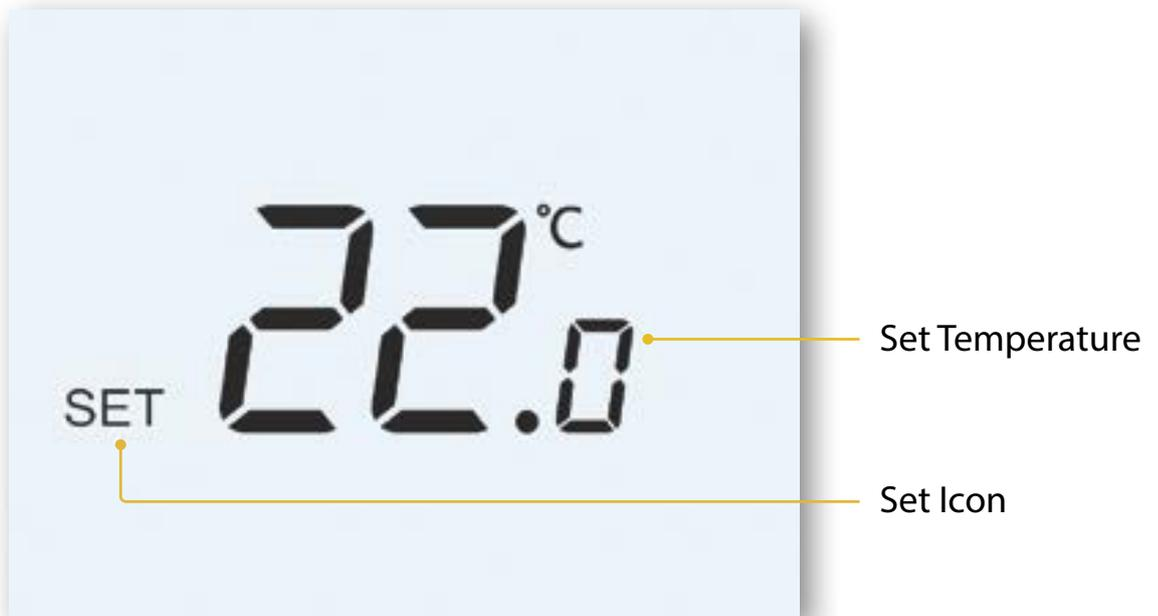
*Note: This new temperature is maintained only until the next programmed comfort level. At this time, the thermostat will revert back to the programmed levels.*
